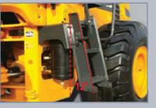
Ladder of Convenience and Safety Tilted ladder by 12 degrees is designed to make getting on and off easier and to enhance comfortability for operators.
