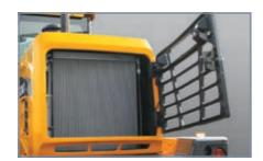
**Easy Access to Radiator** Operators can easily maintain and clean the radiator.
