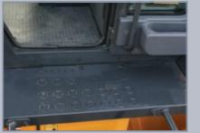
**Non-slip Platform** Non-slip platform and steps ensure operator's safety.
