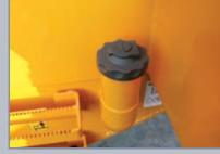
**Key-Locking Fuel Cap** The location of fuel cap increased accessibility and key locking function is applied for machine protection.
