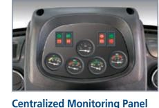
Centralized monitoring panel designed with simplicity of ergonomics that shows working conditions and warning lights at a glance.
