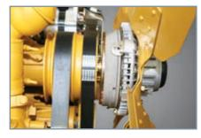
Fan clutch (SL760 only) Fan's speed is adjusted by temperature to reduce engine fuel consumption and noise. Engine durability is increased by warming up engine quickly.
