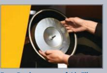
**Easy Replacement of Air Filter** Air filter is built in the rear of the hydraulic tank to ease replacement and cleaning of the filter.
