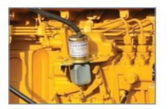
Electric Shut off (SL760 only) When the circuit key turns to off, it stops electromagnetic and closes the throttle.
